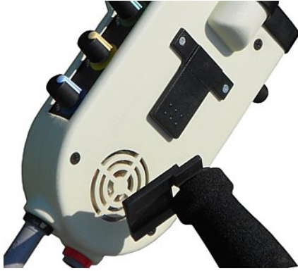
Illustration 4.4: Shows the control unit ready to mount to bracket
