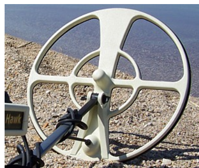
Illustration 4.7: Search Coil mounted to Telescopic Rod
