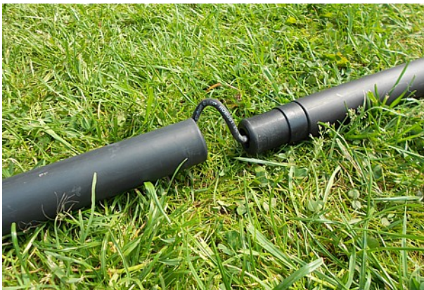
Illustration 4.10: create a loop in the cable to insert into straight pieces
